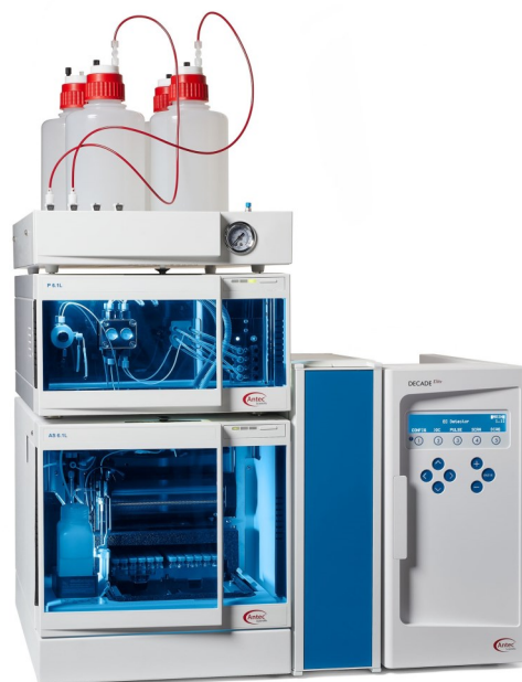
Figure 3. Recommended HPAEC-PAD instrument configuration for this application: the ALEXYS Carbohydrate Analyzer. The system consists of an ET210 Eluent tray for nitrogen blanketing, a P6.1L quaternary LPG pump capable of running gradient program, an AS6.1L autosampler, a CT2.1 column thermostat, and a DECADE Elite electrochemical detector. The ALEXYS Carbohydrate Analyzer can be fully controlled by different Chromatography Data System (CDS) software, namely DataApex™ Clarity™ CDS (version 8.3 and up) or Thermo Scientific™ Chromeleon™ CDS (version 7.2 SR5 and up).
